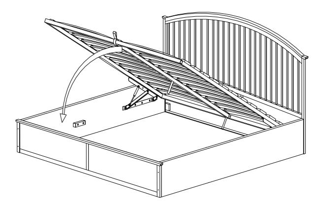
Lift with the strap (H12) and close with the strap. The strap should always be accessible. Take care not to lean over the bed when lifting, if the mattress is thin and light, the frame may rise quickly. The speed of closing will also depend on the weight of the mattress so always keep fingers well clear of the metal frame.
