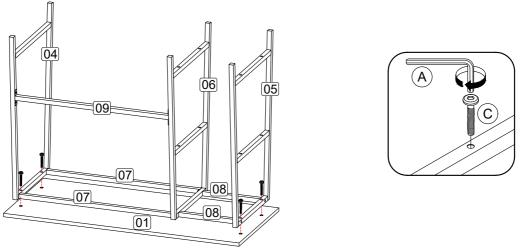
Step 4: Attach the Metal Side Right (5) and Metal Center (6) to panel (2) using hardware A and C. Attach the Metal Side Right (5) and Metal Center (6) to panel (3) using hardware A and C. DO NOT tighten all the screw.
