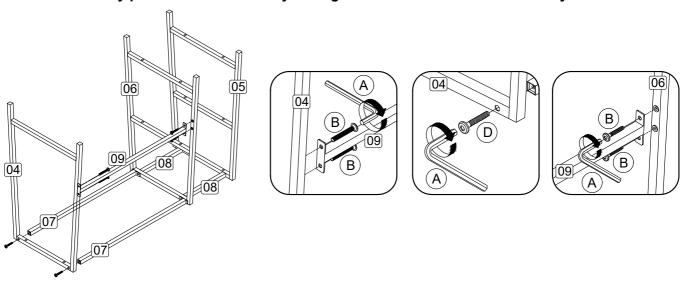
Step 3: Attach the Metal Side Left (4) and Metal Side Right (5) to panel (1) using hardware A and C. DO NOT tighten all the screw.
