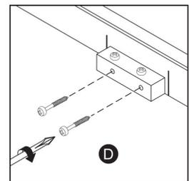
**Step 2:** Insert the left panel (3) to the left front frame (7) making sure the parts are fully pushed together and lined up. Place the cleats (17) between the marks shown and secure using hardware part D and a screwdriver (not provided).
