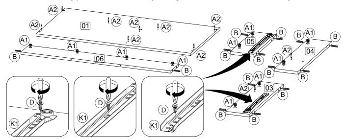
Step 2: Attach the panel (5) and (6) to panel (1) using hardware A1 and A3 with a screwdriver (not provided).
