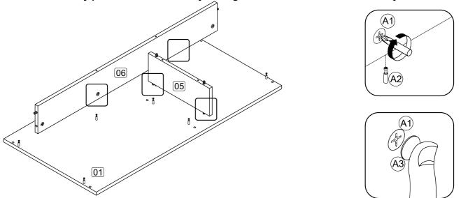
Step 3: Attach the panel (3) and (4) to panel (1) and (6) using hardware A1 and A3 with a screwdriver (not provided).
