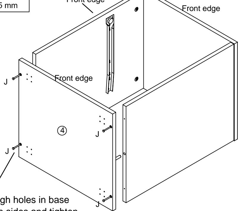
Insert all screws through holes in base into pre-drilled holes in sides and tighten.
