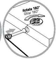
Turn minifix cams to the right to tighten.
