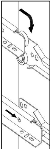
Angle the drawer slightly to ensure that the wheel at the back of the drawer slide goes behind the front wheel on the cabinet slide. Then lift the drawer up and slide it into the channel of the drawer slide.
